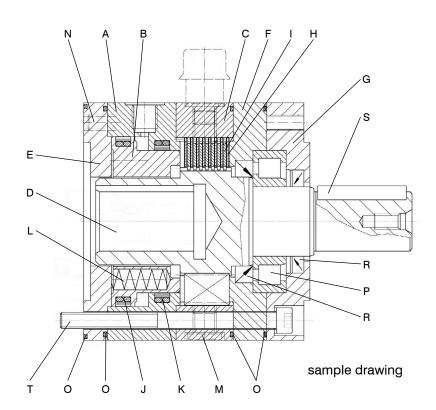
LBD brakes are designed as holding brakes for dry or wet operation.
