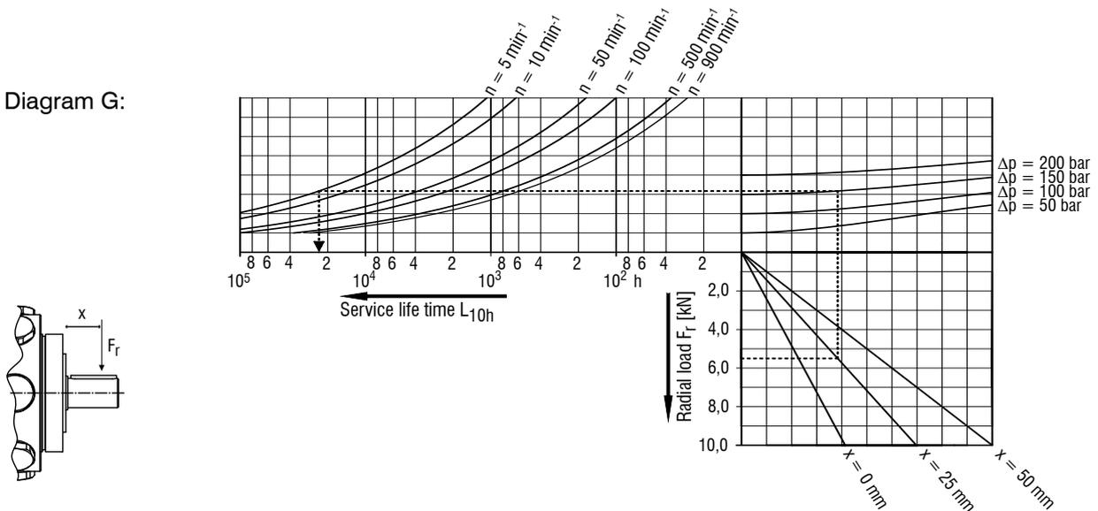
**Given** :  $F_r = 5,5$  kN  $x = 25$  mm  $\Delta p = 150$  bar  $n = 5$  min $^{-1}$
