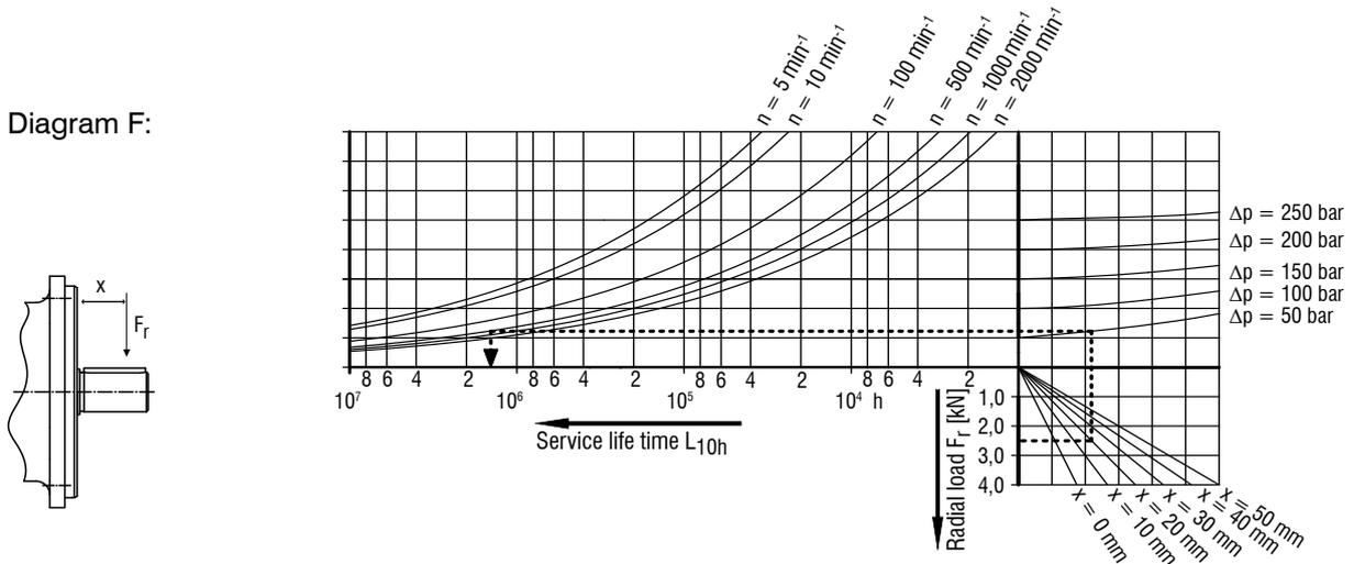
**Given** :  $F_r = 2,5 \text{ kN}$     $x = 20 \text{ mm}$     $\Delta p = 50 \text{ bar}$     $n = 500 \text{ min}^{-1}$
