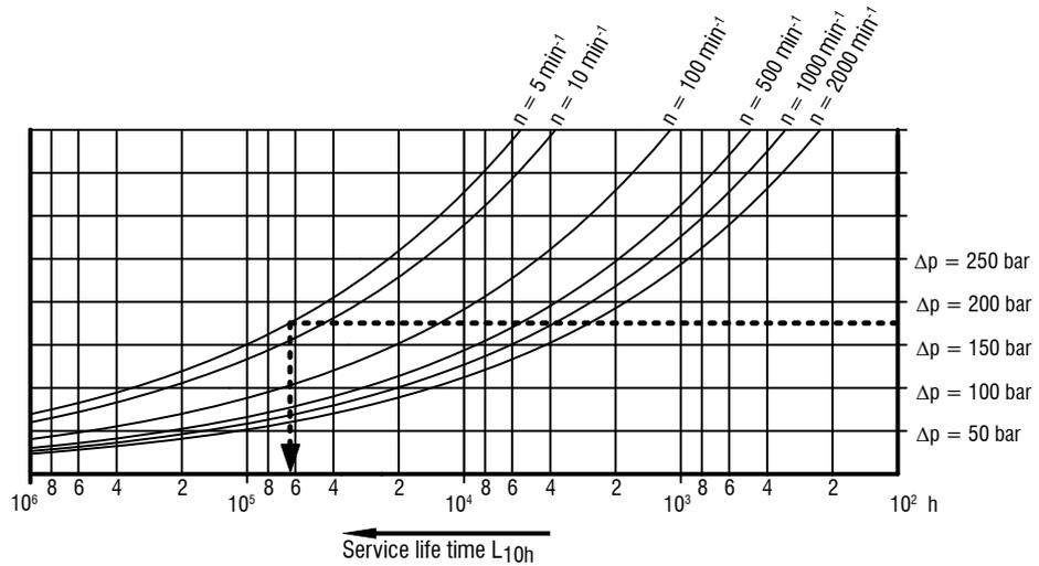
**Given** :  $F_r = 0 \text{ kN}$     $x = 0 \text{ mm}$     $\Delta p = 175 \text{ bar}$     $n = 5 \text{ min}^{-1}$
