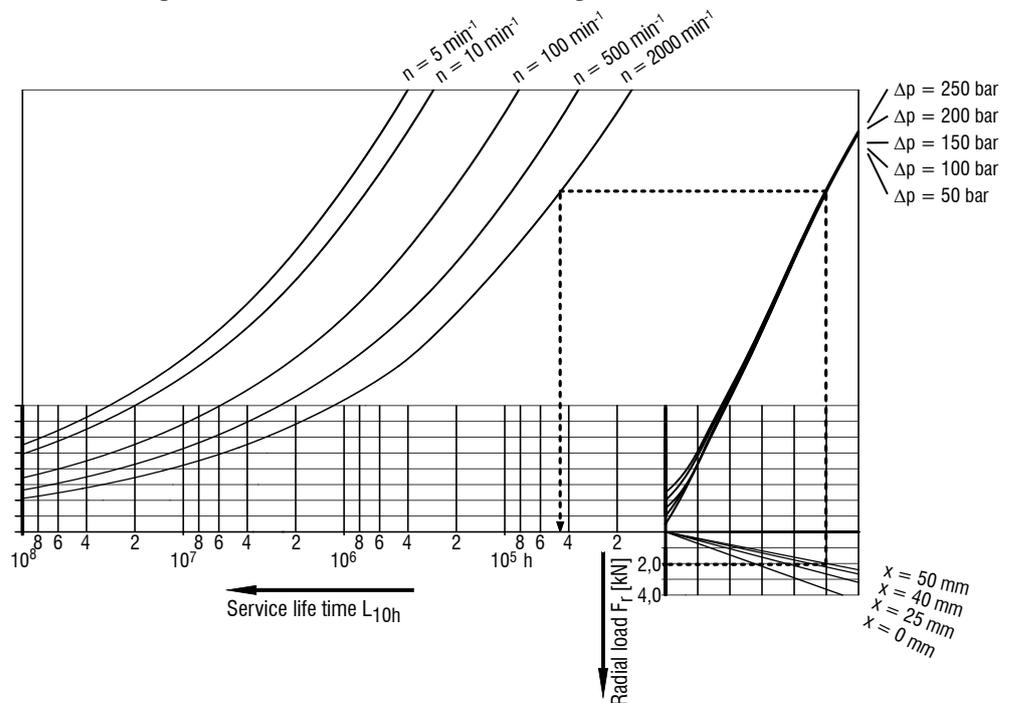
**Given** :  $F_r = 2 \text{ kN}$     $x = 50 \text{ mm}$     $\Delta p = 100 \text{ bar}$     $n = 2000 \text{ min}^{-1}$
