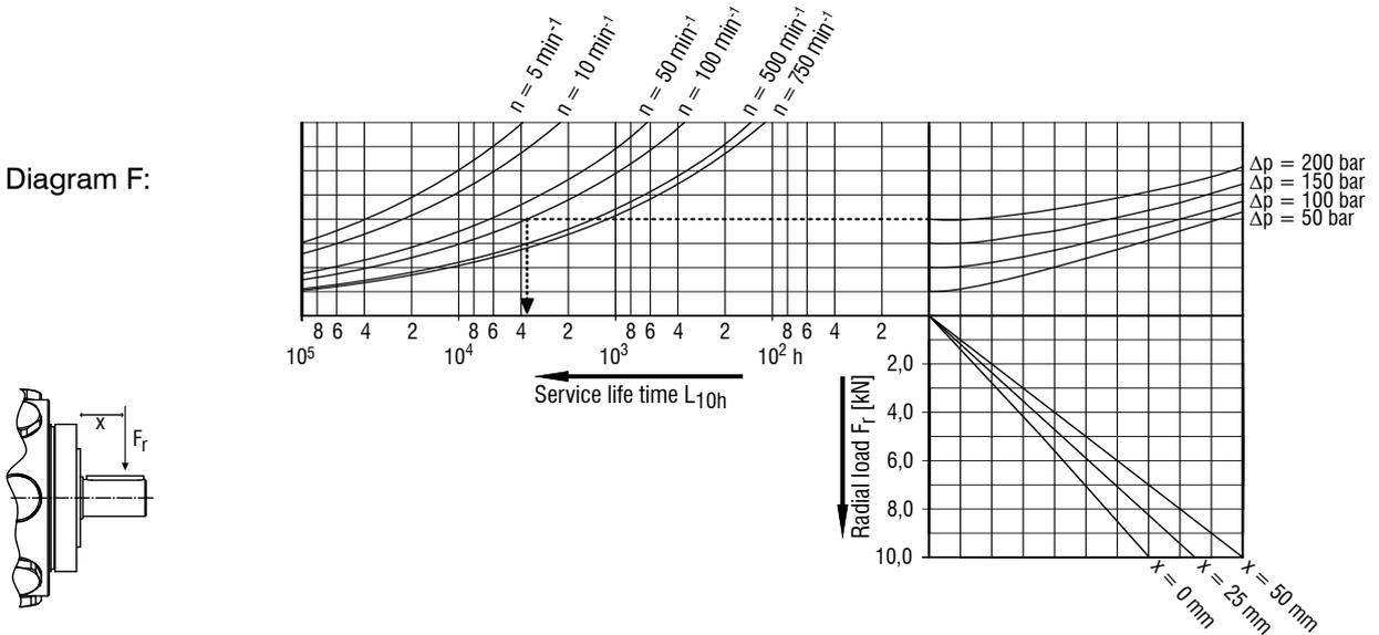
**Given** :  $F_r = 0$  kN  $x = 0$  mm  $\Delta p = 200$  bar  $n = 100$  min $^{-1}$
